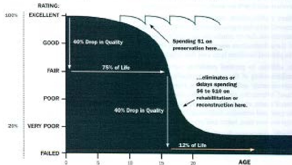
Figure 6: Example of asset deterioration curve (Roads)
